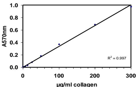
*A typical collagen standard curve in the range of 6 - 300  $\mu\text{g}/\text{ml}$  collagen.*
